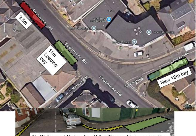
No Waiting and No Loading At Any Time restriction on junction
