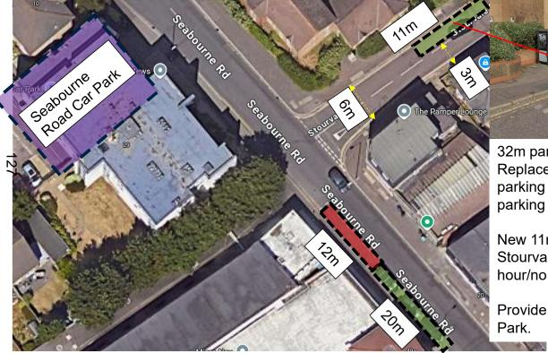
32m parking section reduced by 12m (approx. 2 vehicles). Replace with 'No Waiting At Any Time' restriction. Remaining 20m parking section retained with no alterations to existing timed parking restrictions.
